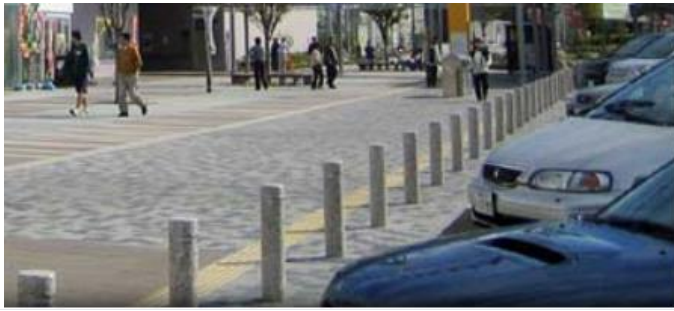
Plate 1. Use of bollards to separate vehicles from intruding into the pedestrian area Source: https://www.bing.com/images/
